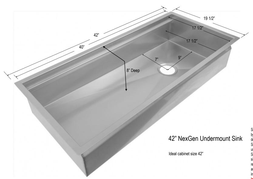
Sink should be supported by flanges only. Sink gets deeper than 8" toward drain. Silicone should NEVER be used with a copper sink! Silicone is fine with stainless sinks. Plumbers putty is recommended with copper and stainless drain/flange installation.
